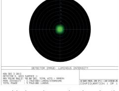
Graphic in polar mode given by the simulator which shows the intensity produced by the LED with the lens. It measures the light projected in a hemisphere, instead of on a plane
